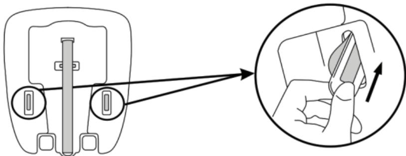
Turn the webbing retainers on their narrowest end and feed them through the slots in the base of the seat and then through the slots in the fabric cover.
