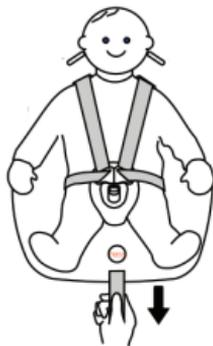
Pull the shoulder straps upwards to remove the slack from the lap sections of the harness, then pull the adjuster strap until the harness is fully tightened.
