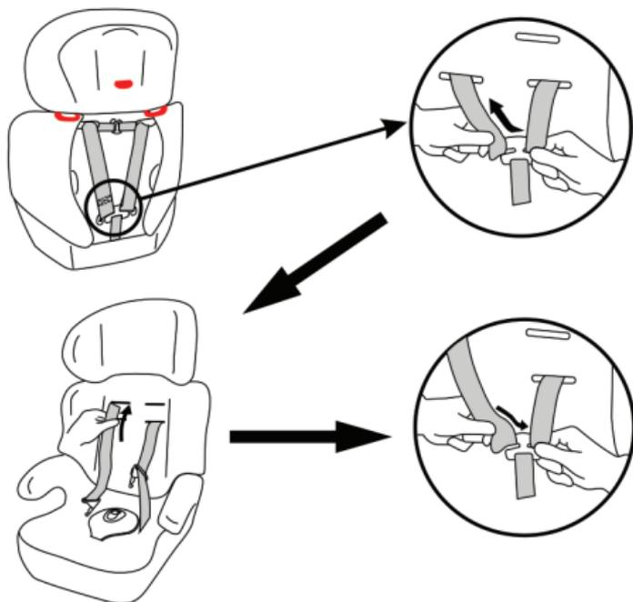
Firstly, release the strap holding the backrest cover on to gain access to the harness. Slide one of the harness straps off the harness connector. Then from the front of the seat, pull it through the slot in the seat's backrest and fabric cover. Thread the harness strap back through the next hole up or down on the seat's backrest.
