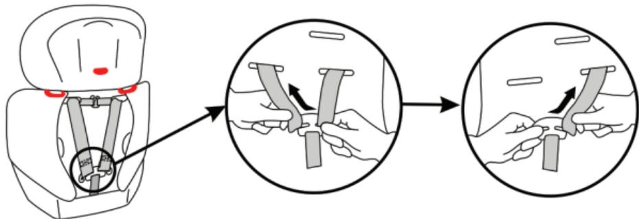
Release the strap at the bottom of the backrest cover to gain access to the harness. Slide both of the harness straps off the harness connector at the back of the backrest and pull the webbing through the slots in the seat's backrest and fabric cover.
