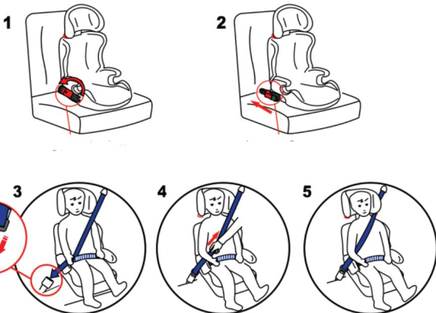
1. Rotate out the Isofix connectors until you hear "Click". Check that the Isofix connector is moving within the angle of 15°, and cannot turn around.
